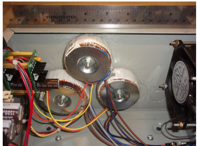
Fig. 8. Transformers (right), power supplies (left), and rotatory joint (bottom).
