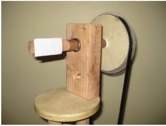
Fig. 10. Roll axis complete with roll pulley, shaft, bearings and belt flange. The shaft is cut longitudinally to allow for easy AUT connection with, for example, double-sided tape, like shown in this figure
