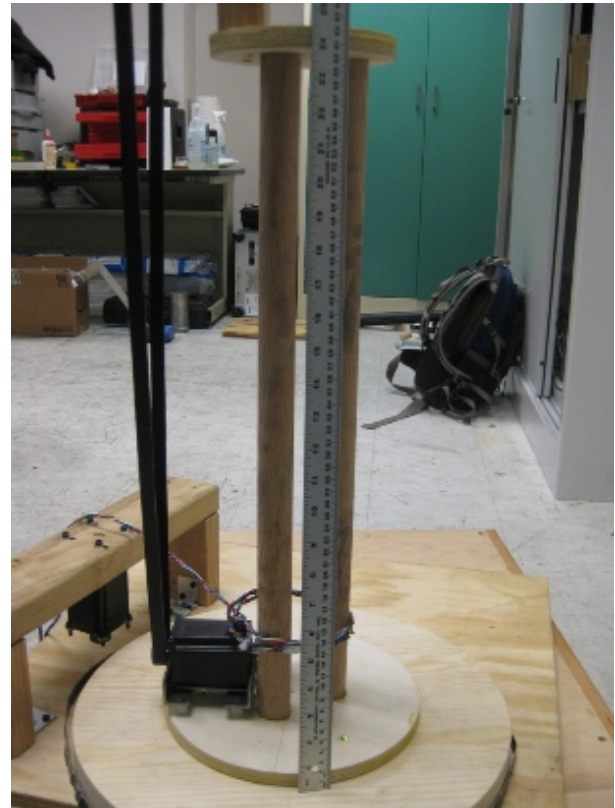
Fig. 9. Column supporting the upper disc and the roll wheel
